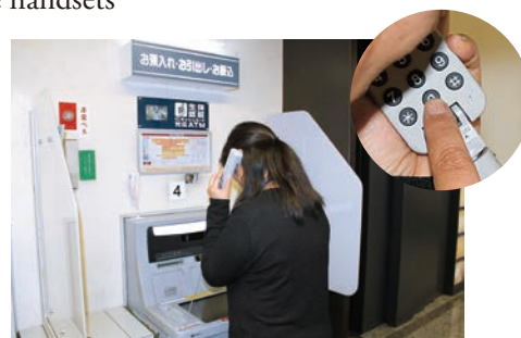
ATMs with audio assistance using phone handsets
